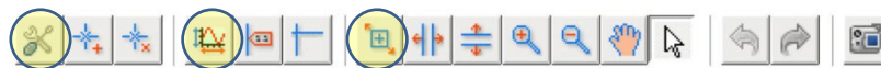
Figure 5. Graph Toolbar, with the Configure Settings, Perform Autoscale and Rubberband Zoom buttons highlighted (left to right).
