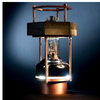
Figure 4.2-1. The world's smallest neutrino detector, a cesium iodide crystal, that discovered coherent elastic neutrino nucleus scattering at SNS.
