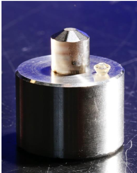
10 carat, 9 mm tall CVD anvil with pyramidal design
