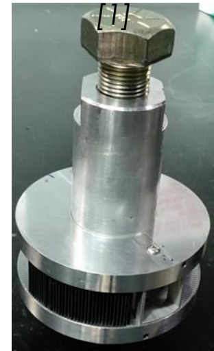
Gas pressure cell with radial SNAP collimator
