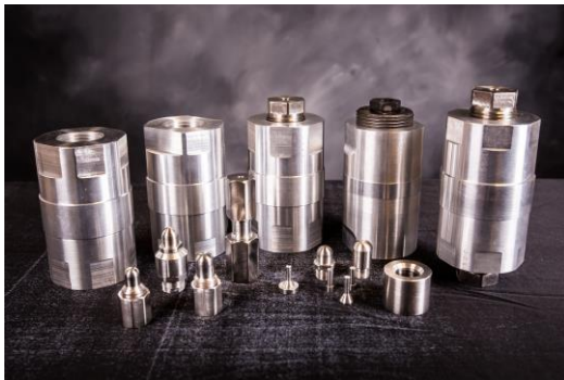
NiCrAl cell that can be cooled to 300 mK and allows maximum pressures of 2.2 – 3 GPa.
