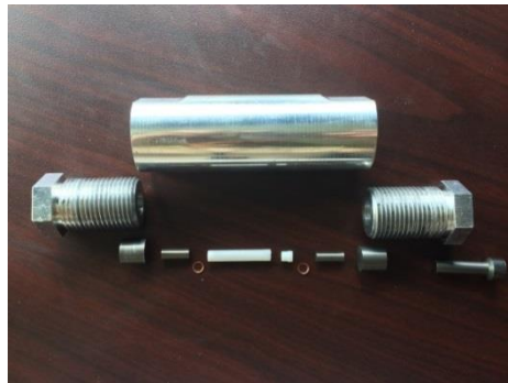
NiCrAl cell that can be cooled to 300 mK and allows maximum pressures of 2.2 – 3 GPa.
