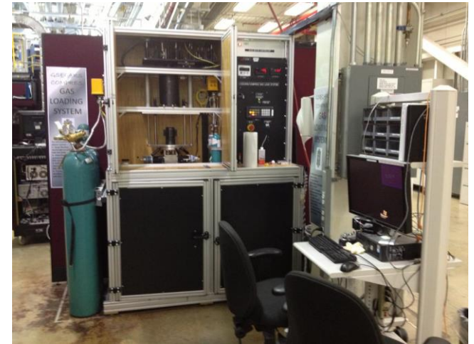
GSECARS/COMPRES gas loader
