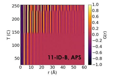
Data collected for 1 µm films deposited **on kapton**, thermally annealed in situ under flowing He to 155°C and measured at ~60 keV in transmission
