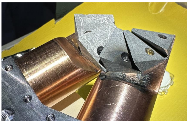
Figure 3: Electron catcher with signs of overheating.
