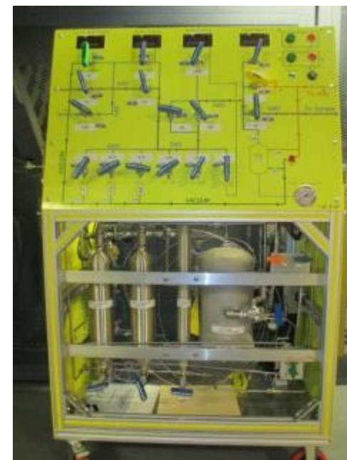
Gas handling panel for gas dosing, mixing, flow, adsorption (vacuum to 200 bar)
