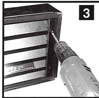
Swing door grill removal. Loosen but do not remove 4 Phillips screws inside the grill frame.
